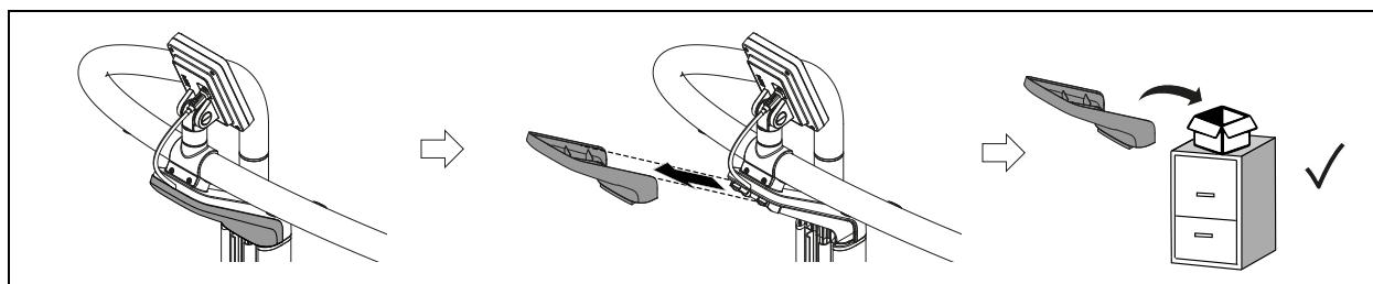
6. ABDECKUNG SÄULE ABNEHMEN • REMOVING COLUMN COVER • ENLEVER LE CACHE DE LA COLONNE •
