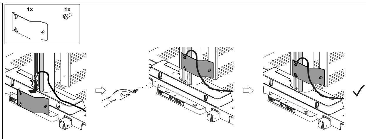
**13. LÄNGENMESSSTAB AN UNTEREN HALTER MONTIEREN • MOUNTING MEASURING ROD TO LOWER BRACKET •
