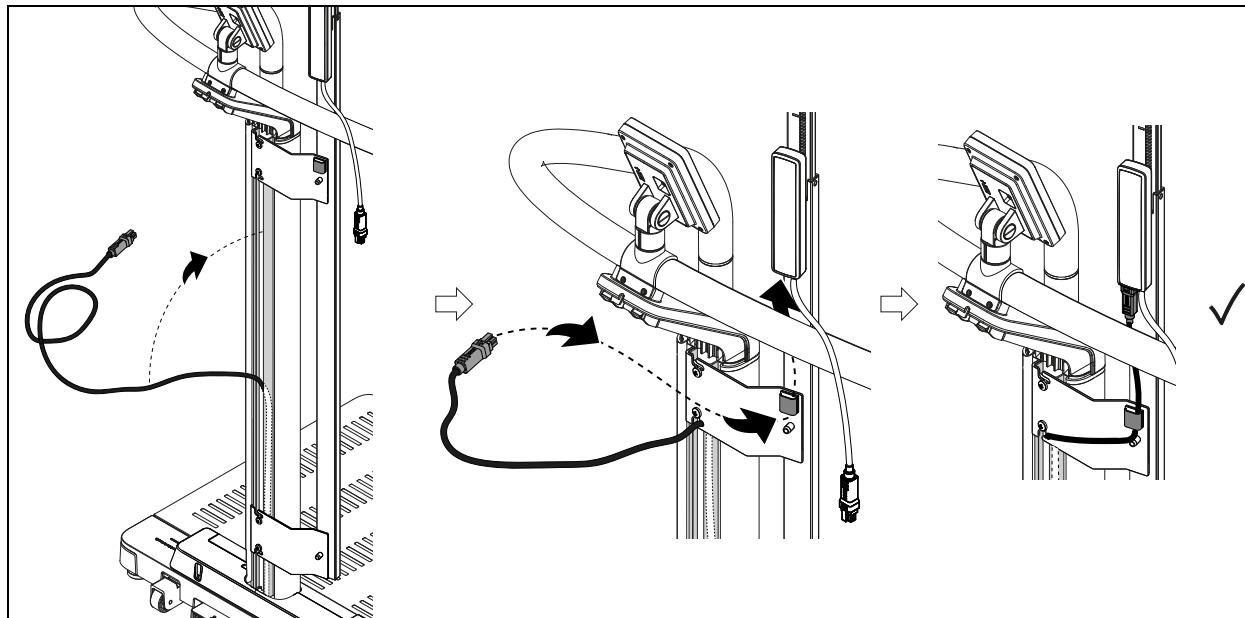
16. MESSSTABKABEL AM DISPLAY ANSCHLIEßen • CONNECTING MEASURING ROD CABLE TO DISPLAY •
