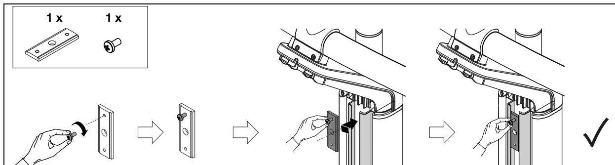
9. OBEREN HALTER MONTIEREN • MOUNTING UPPER BRACKET • MONTER LE SUPPORT SUPÉRIEUR • MONTAR EL SOPORTE SUPERIOR
