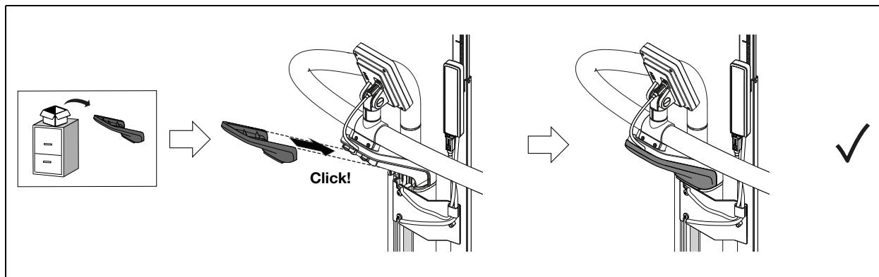
**18. SÄULENABDECKUNG AUFSETZEN • PLACING COLUMN COVER • POSITIONNER LE CACHE DE LA COLONNE • COLOCAR LA CUBIERTA DE LA COLUMNA**
