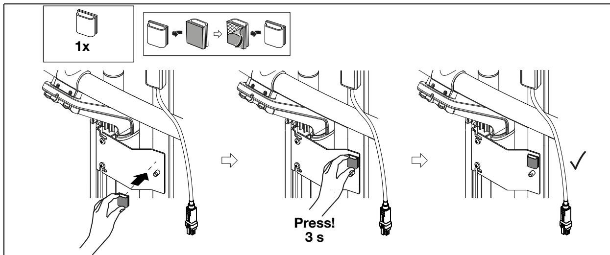
15. DISPLAYKABEL AN MESSSTAB ANSCHLIEßen • CONNECTING DISPLAY CABLE TO MEASURING ROD •
