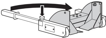
**Route cable so that it is not in contact with the grey parts shown in the drawing.**
