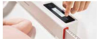
The digital measuring rod simplifies the measuring process with its large display and transmission function.
